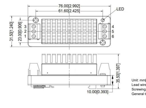
Unit: mm[inch] Lead wires size: 24-12AWG Screwing torque: 0.4N.m Max General tolerance ±1.00[±0.039]
