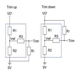
Rrim Resistance calculating fomulaup: $RT = \frac{\alpha R_2}{R_2 - \alpha}$  $-R_3$  $\alpha = \frac{Vref}{Vo' - Vref}$  $R_1$ down: $RT = \frac{\alpha R_1}{R_1 - \alpha}$  $-R_3$  $\alpha = \frac{Vo' - Vref}{Vref}$  $R_2$
